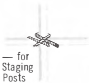
As a Strong Crossing Knot in Lashing Heavy Parcels
